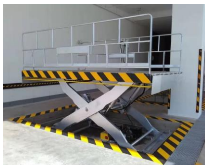
Scissor lift (Lever, screw, toothed bar)
